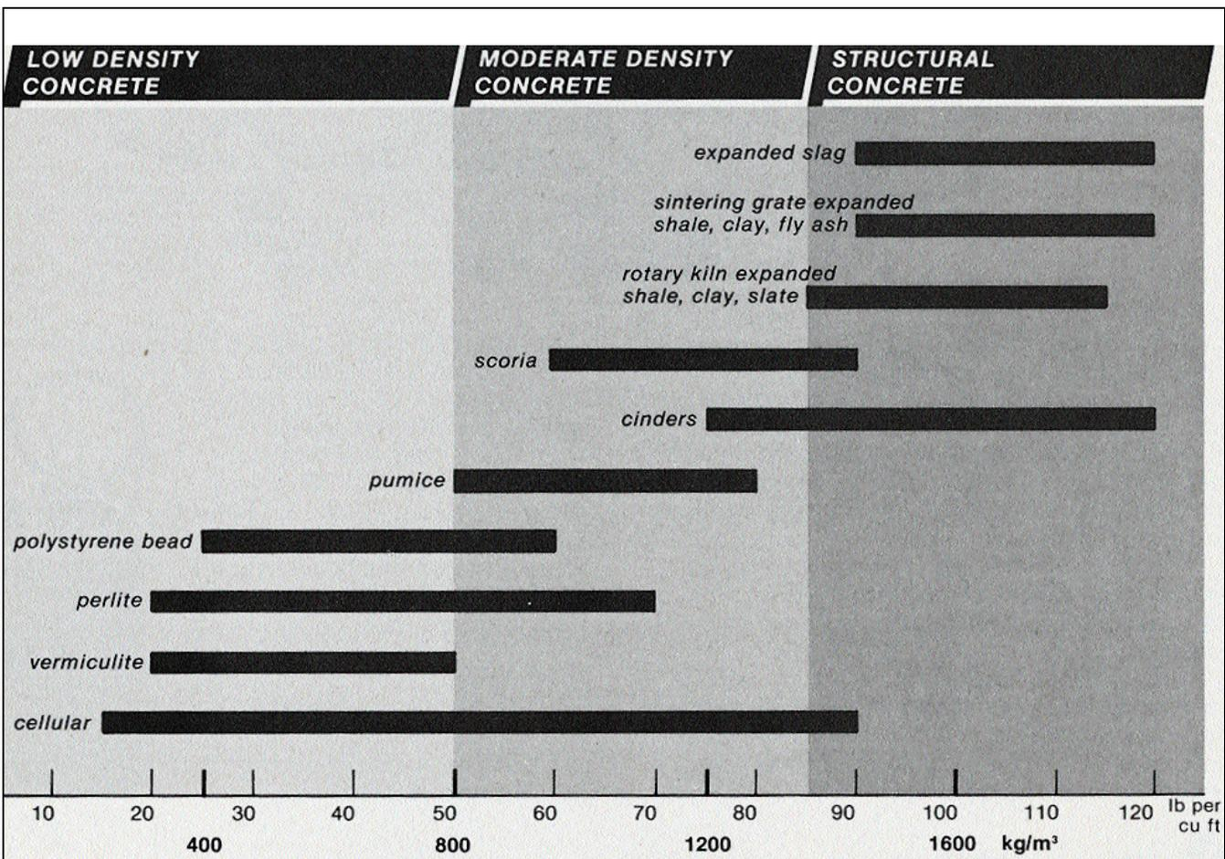
Air-dry densities of lightweight concrete range from 12 to 120 pounds per cubic foot. Structural lightweight concretes at the right end of the spectrum have strengths of 2500 psi and above. Adapted from ACI 213R-79, Reference 1.
